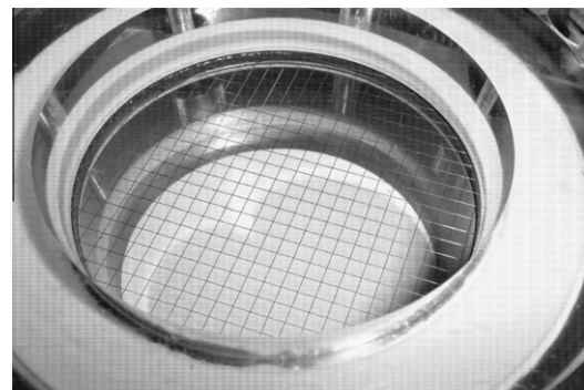
Fig. 3. Photograph of the 24 \times 24 wire mesh sensor.
