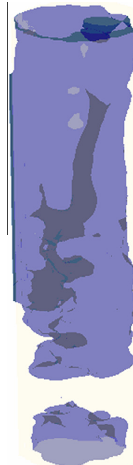
Fig. 14. Interface between wall film and gas and gas and central liquid structure. Gas superficial velocity = 5.7 m/s; liquid superficial velocity = 0.25 m/s.
